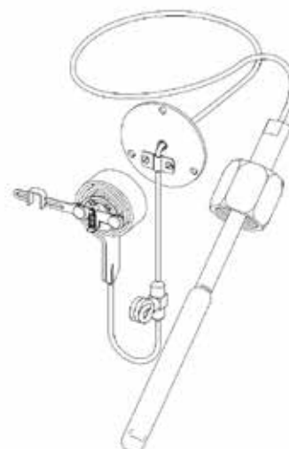
Temperature-sensing nitrogen-filled, 2 m capillary length, conn. 3/4" GAS, bulb for liquids, material: S.S. ASTM A240 Type 316L.
